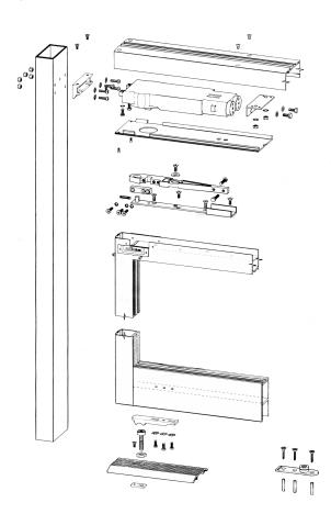
The set of door controls comprises three main items. Firstly, a sealed unit 'the closer body' which is fitted inside the transom bar above the door and concealed with a removable cover plate. Secondly, a steel drive arm with a steel fixing channel fitted
