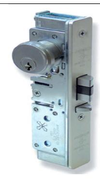
A reverse turn of the key (while bolt is held fully retracted) retains the bolt, allowing the door to be free swinging.
